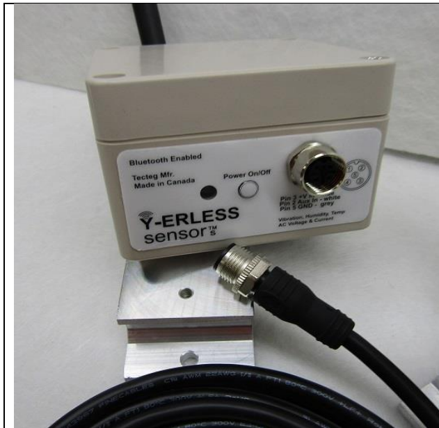
Front panel showing the 5 pin mini connector for power attachment for either battery or industrial power connection or energy harvesting.
