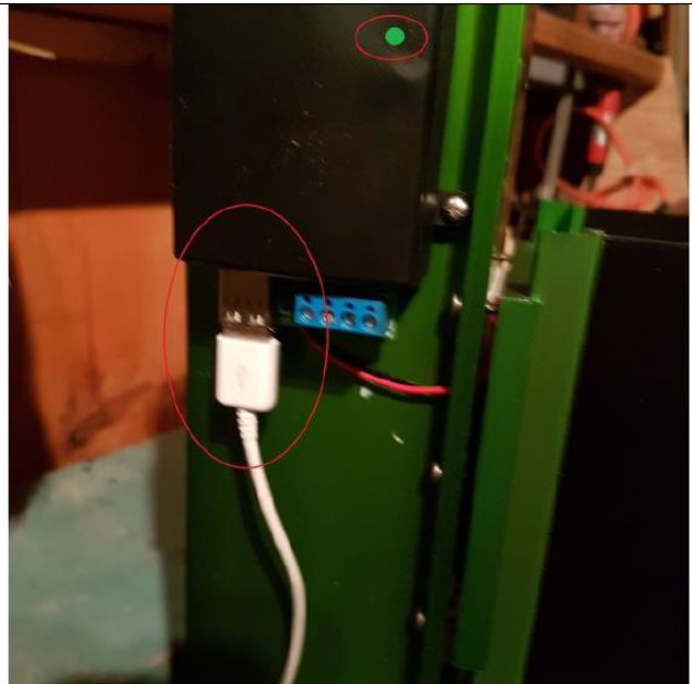
13) Once the green light is on. Connect your cell phone with its charger cable to the USB port. If you are using an iPhone you will need to use the adapter. If the phone is not charging then make the flame a bit bigger.
