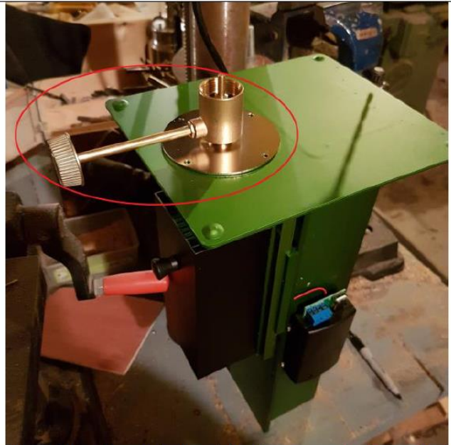
2) Turn the unit upside down and place the burner on it. You may have to prop the unit against something.
