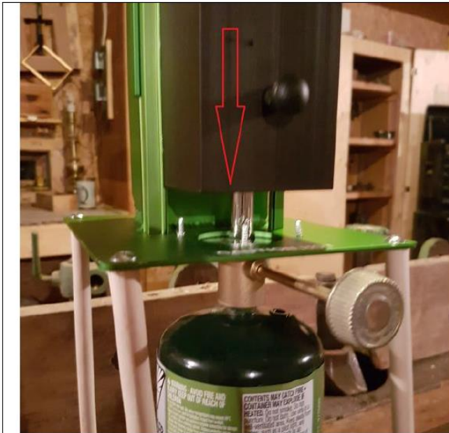
12) Move the flame shield down so that the flame is covered for safety reasons.
